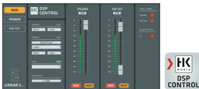
Screenshot of the remote DSP CONTROL software. You can download this software from the DSP CONTROL software download page at www.hkaudio.com . The speaker and DSP Out parameters are identical, but the double DSP power lets you configure each set independently.
